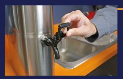
Replace spigot with new pinch-tube spigot.
