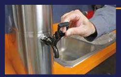
Replace spigot with new pinch-tube spigot.
