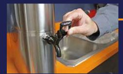
Replace spigot with new pinch tube spigot. Open spigot.
