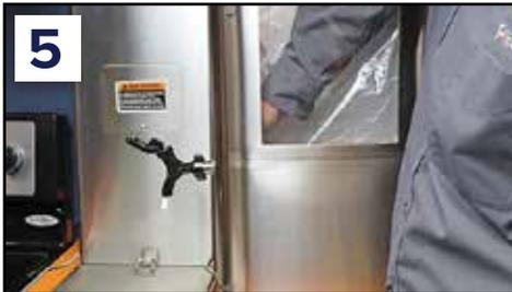
**5** Feed the white tube into the hole in the bottom of the urn until the tube protrudes through the spigot on the outside of the urn.
