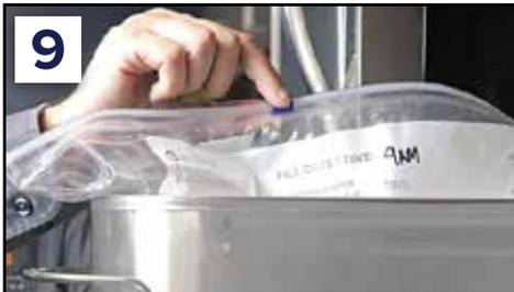
**9** Slide the blue zip locking tab from side to side to seal the liner. Do not pull up on the blue tab as this may cause it to detach.
