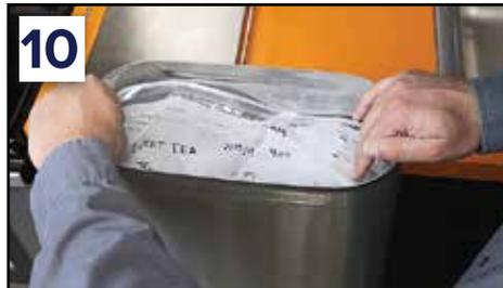
**10** Fold the top of the liner over with the label clearly visible and replace urn lid.
