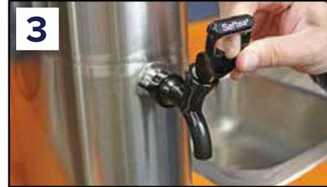
**3** Open the Saftea® pinch tube spigot. (The “open” position is pulled fully forward & down.)
