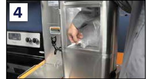
**4** Place liner into urn. Always handle liner from the outside to keep it contaminate free.
