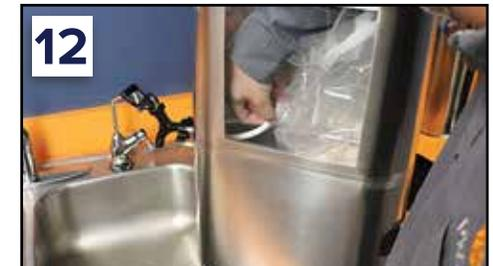
**Removal:** Open spigot, reach into urn, pinch & pull the white tube out of the bottom of the urn. Discard or recycle liner. Remove tube before recycling.
